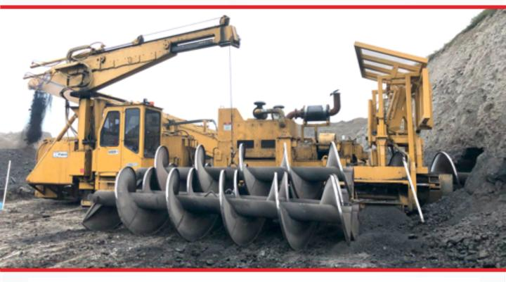
**AUGER MINING** is a surface mining technique used to recover additional coal drilling into the exposed coal seam at the limit of surface operations.
